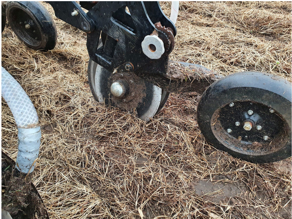
Figure 18. Close-up of Gent® double disk opener and press-wheel giving zero soil disturbance and maximum soil protection. This planting machinery was evaluated on-farm across a range of sites as part of the 'Legume Project'. Planter sponsored by Direct Seeding. https://directseeding.com.au/
